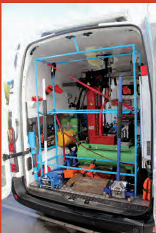
Let the sunshine in: Solar panels on the roof power the gear for changing tyres inside, including Nitrogen generator, middle. Rack in the back allows the van to make more than one call.
