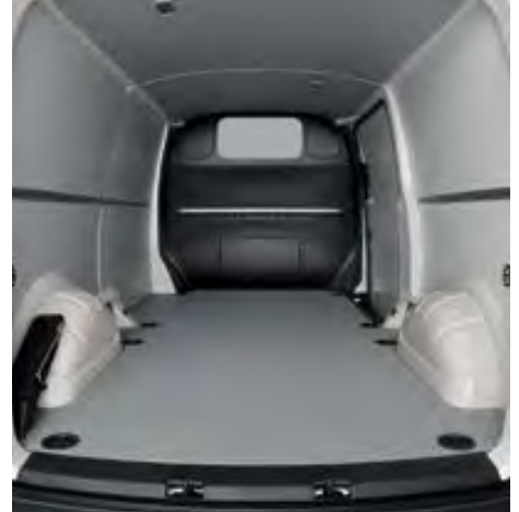
Optional fixed partition with fixed window and wooden floor. Overseas model shown.
